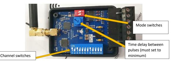
The red DIP switches on the transmitter must both be set to OFF
